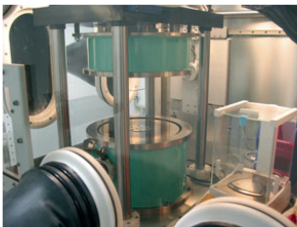
Fig. 1: The reaction chamber of the SPS-system inside the glove box.
